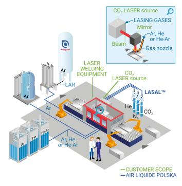
Designed for laser welding with all types of sources, **LASAL™ SHIELD NOZZLE** improves shielding gas distribution in the interaction zone. This solution contains gas jet dispersion at the nozzle's end, achieving the highest possible laminar flow above the weld pool.
